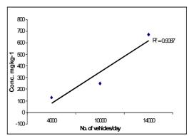
Fig. 11: Correlation of Zn levels in surface soils with traffic density
