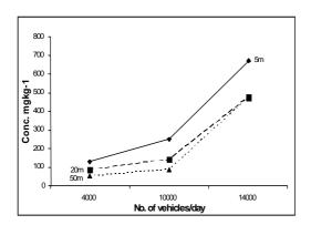
Fig. 10: Zn levels in surface soils in sections A, B, C
