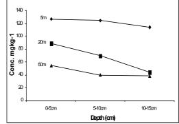
Fig. 8: Zn levels at various distances and depths in section B
