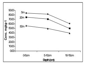
Fig. 13: Cu levels at various distances and depths in section B
