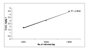
Fig. 21: Correlation of Cd levels in surface soils with traffic density
