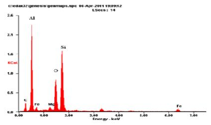
Fig 2: SEM analysis of elemental composition of aluminum alloy (matrix)
