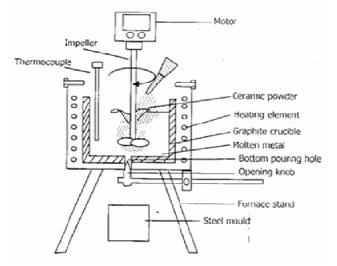
Fig. 3: Schematic diagram of stir casting technique
