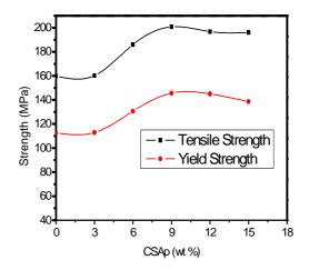
Fig. 7: Variation of strength with wt% coconut shell ash particle
