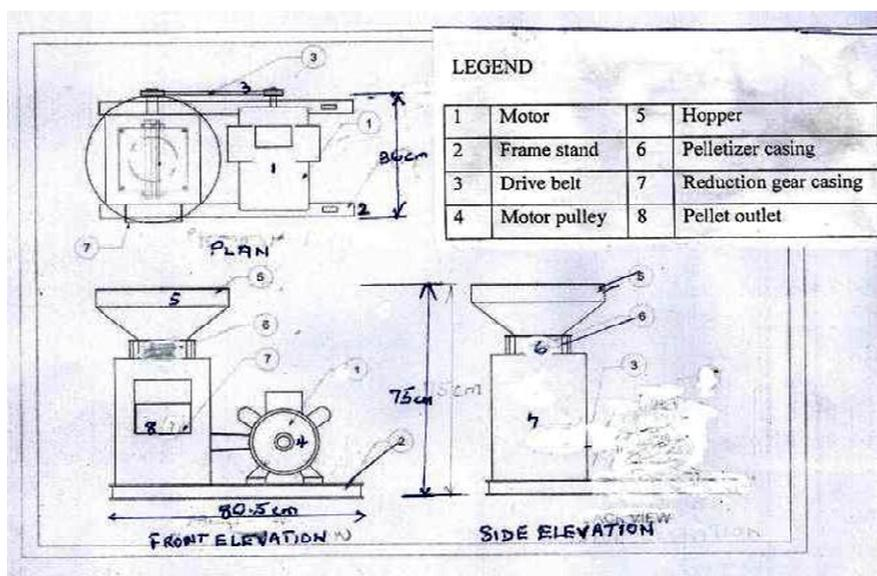
**Fig. 4: The designed and fabricated fish meal pellet machine**
