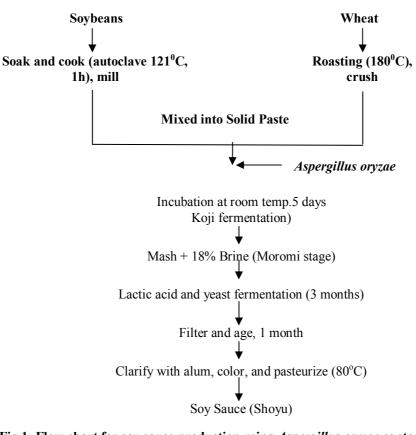
Figure 1 shows the flow chart for the production process of soy sauce
