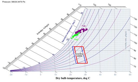
Fig.1: Mean hourly temperature and relative humidity values in Kumasi for representative days in the months of February and August (based on data generated via Meteotest (2008)
