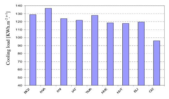
Fig.12: Simulated cooling loads (DCD) for different scenarios (see Tables 3 and 4)
