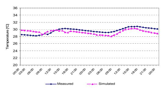
Fig.7: Measured versus simulation indoor air temperatures in KCR
