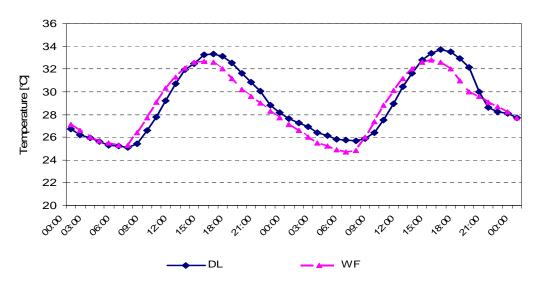
Fig.5: Outdoor air temperatures from weather file segments (WF) used for simulation calibration in comparison with measurements (DL) at building location (DCD)
