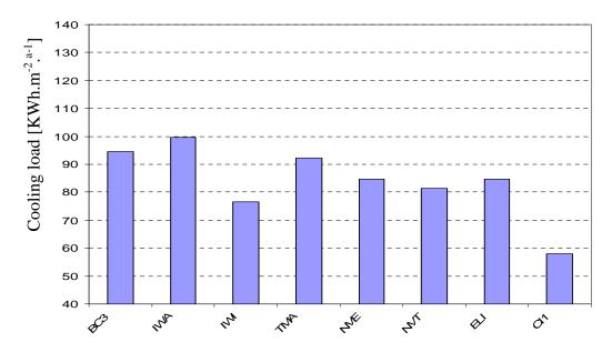
Fig.11: Simulated cooling loads (ROY) for different scenarios (see Tables 3 and 4)
