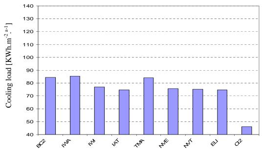
Fig.9: Simulated cooling loads (KCR) for different scenarios (see Tables 3 and 4)
