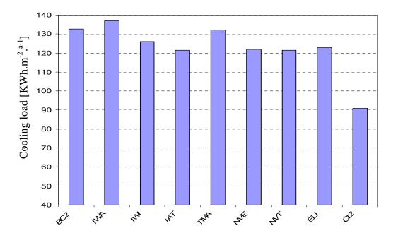
Fig.10: Simulated cooling loads (ANG) for different scenarios (see Tables 3 and 4)
