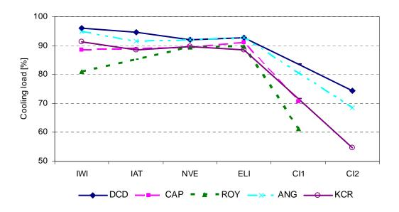
Fig.13: Simulated cooling loads (in percentage of the respective base cases) for all buildings and for selected scenarios (see Tables 3 and 4)
