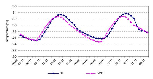
Fig.4: Outdoor air temperatures from weather file segments (WF) used for simulation calibration in comparison with measurements (DL) at building location (ANG)
