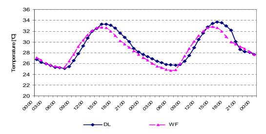
Fig.3: Outdoor air temperatures from weather file segments (WF) used for simulation calibration in comparison with measurements (DL) at building location (KCR)
