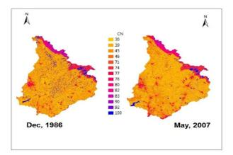
Fig. 8: Curve number map for Barekese catchment area
