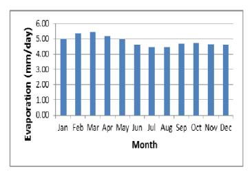
Fig. 12: Estimated average monthly evaporation for Kumasi using the Penman Evaporation Model (2001-2010)
