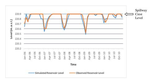
Fig. 14: Simulated and observed reservoir levels for the validation period (2006-2010)
