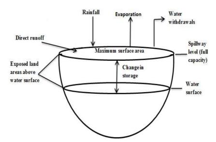
Fig. 3: Schematic view of the water budget of Barekese Reservoir (adopted from Yeung, 2005)
