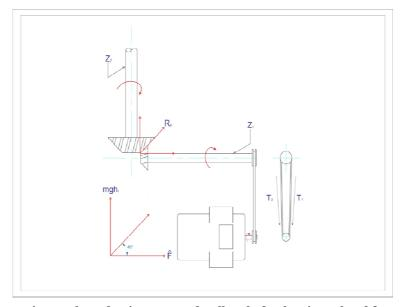
Fig 3: Forces acting on the reduction gear and pulley shafts showing related forces and direction
