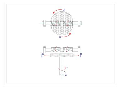
Fig 2: Centrifugal force on perforated disc, angular rotation of disc and roller cutter
