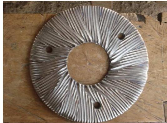
**Fig. 1: Locally-manufactured corn-mill plate.**
