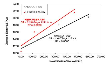
Fig. 15: Change in Acoustic Energy and Area of Delamination for Feed Rate of 1 mms<sup>-1</sup>
