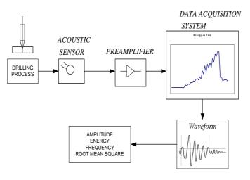
Fig. 3: Schematic Showing Experimental Set-Up
