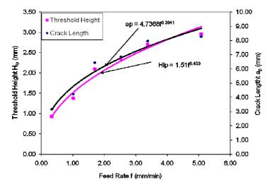
Fig. 6: Longitudinal Crack Length/Threshold Height versus Feed Rate for Amoco T300
