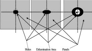
Fig. 12: Relationship between Tool Size and Crack Dimensions
