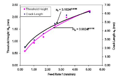
Fig. 7: Longitudinal Crack Length/Threshold Height versus Feed Rate for Hercules AS4
