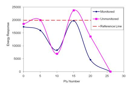
Fig. 18: Energy Response versus Ply Number @ speed of 1000 mm/min for Hercules AS4
