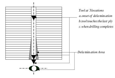
Fig. 2: Formation of Delamination Cracks
