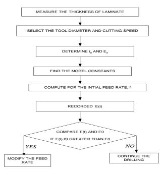
Fig. 16: Implementation of the Selection Monitor of the Drilling Process
