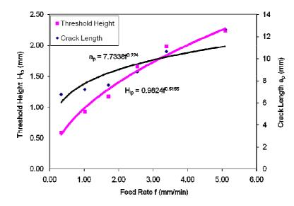
Fig. 10: Transverse Crack Length/Threshold Height versus Feed Rate for Hercules AS4
