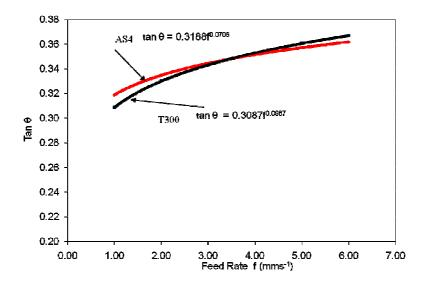
Fig. 8: Tangents of the Inclined Crack Growth Angle  $(\theta)$  and the Feed Rates
