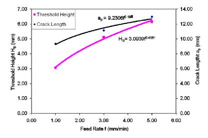
Fig. 9: Transverse Crack Length/Threshold Height versus Feed Rate for Amoco T300
