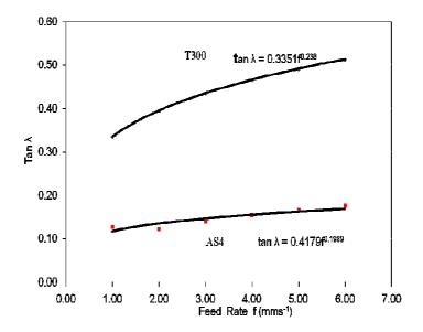
Fig. 11: Tangents of the Crack Growth Angle ( $\lambda$ ) and the Feed Rates
