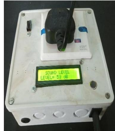
c: SLMC device @  $L_{eq} < 55\text{dB}$
