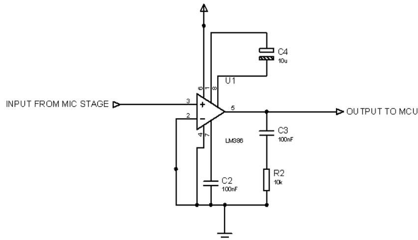
**Figure 3:** Microphone amplifier stage
