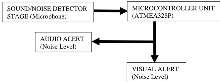
**Figure 1:** Design stages of the developed device
