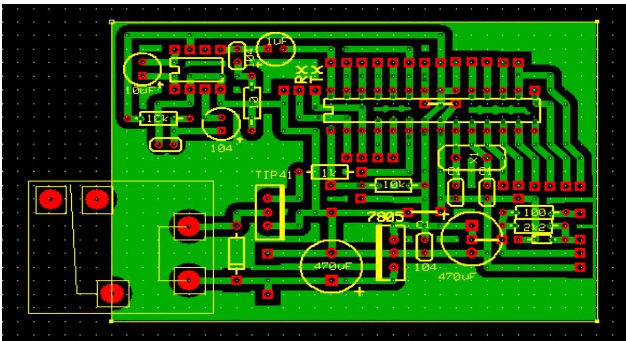
Figure 4: PCB artwork for the design of the noise level monitoring system
