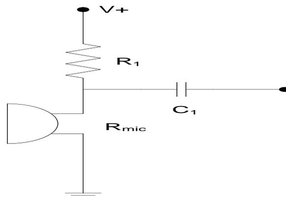
**Figure 2:** Microphone stage
