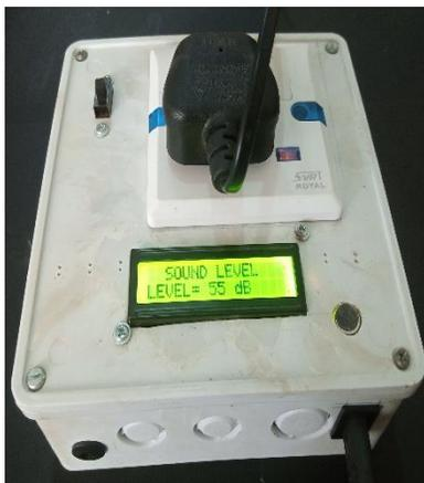
d: SLMC device @  $L_{eq} = 55\text{dB}$
