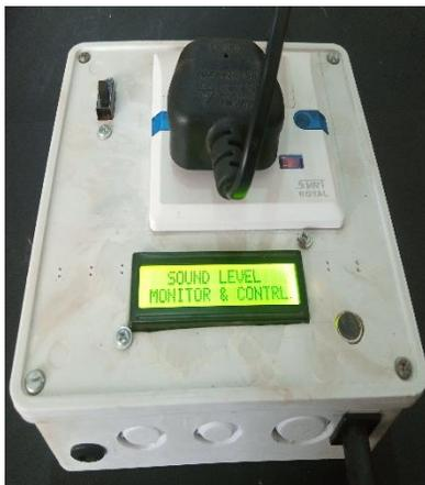
a: SLMC device when switched on
