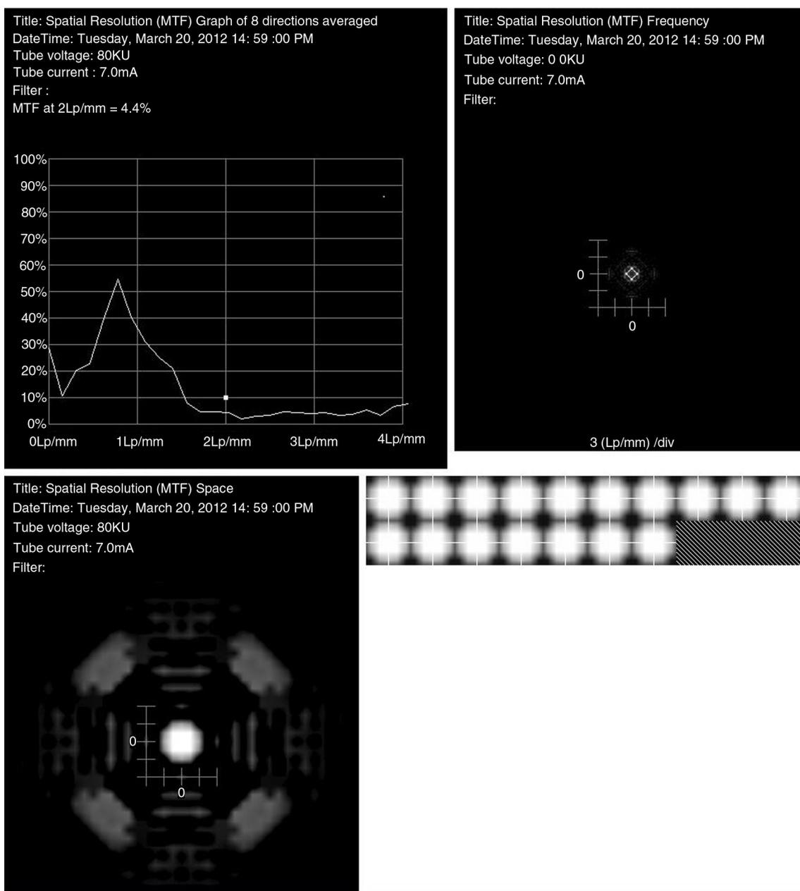
*Fig. 5.* MTF in 3D Accuitomo (60 × 60, 80 kv, 7 mA) to be 4.4% when set at 2 lp/mm (upper left panel). The object on which MTF value was assessed had a spatial frequency of 3 lp/mm (upper right panel) in the space inside the phantom (lower left panel). Axial slices of the object show the luminance intensity after receiving the X-ray signal; no artifacts were noticed (lower right panel).
