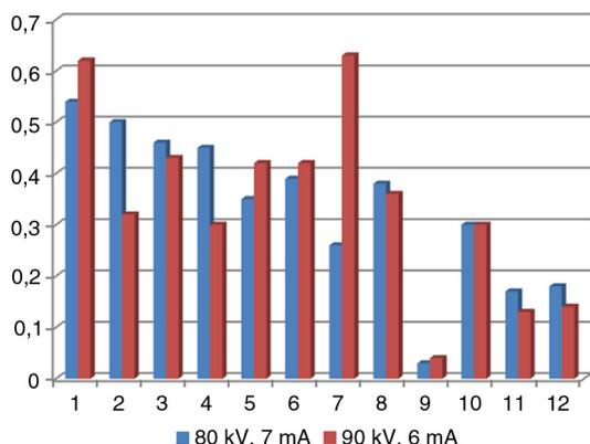
Fig. 9. The graphic distribution of the radiation doses in the two scans of 3D Accuitomo 80. It can be seen that the values in the two scans are generally similar and, using paired *t*-test, no significant differences were found ( $p > 0.05$ ).
