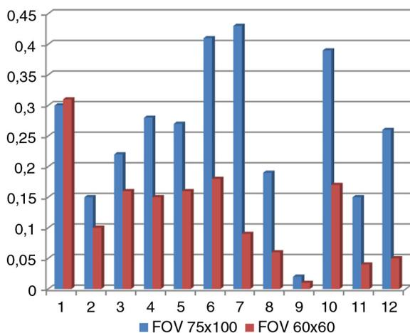
Fig. 10. The graphic distribution of the radiation dose value of the Scanora 3D in the two sessions of changing FOVs. It is obvious that the values of the wider FOV (75 × 100) tend to be higher than the 60 × 60 FOV ( $p < 0.05$ ).
