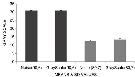
**Fig. 6.** A graph illustrating the means of grayscale values and SD value of the central region (for noise) in both measurements. The SD is shown as small vertical bars on the smaller columns, while the SD of longer columns was zero: 90 = 90 kV, 6 = 6 mA, 80 = 80 kV, 7 = 7 mA.
