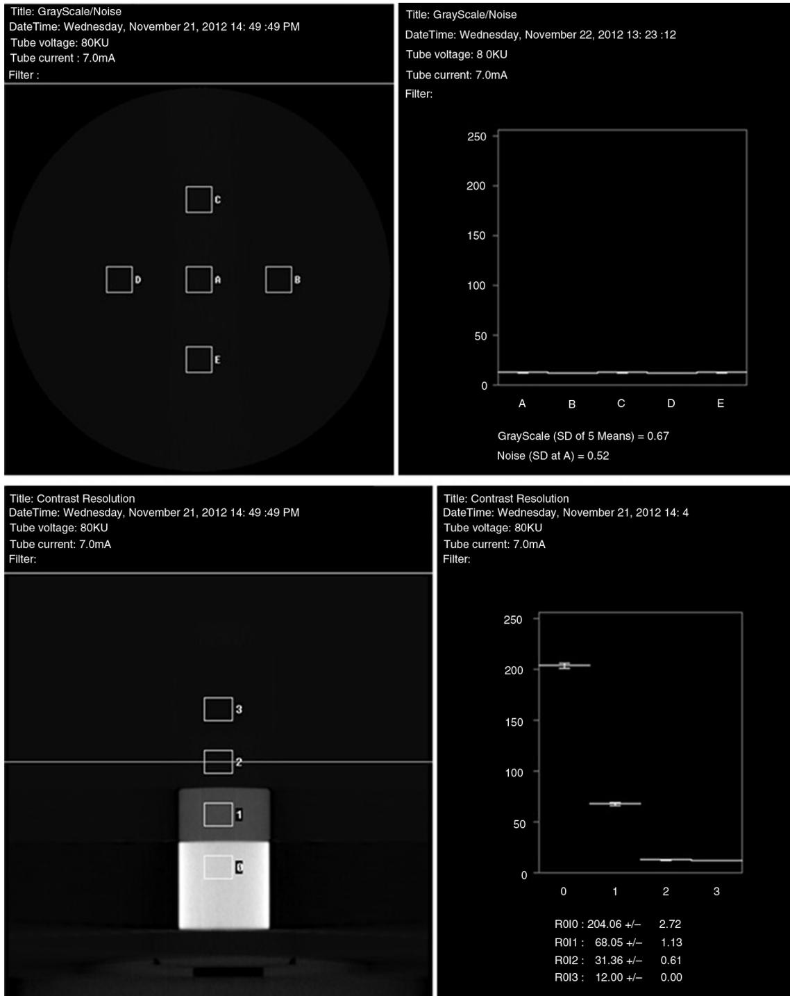
**Fig. 8.** Contrast measurement in 3D Accuitomo 80 (60 × 60, 80 kv, 7 mA) showing uniformity/grayscale of five selected regions in the phantom (upper left panel), and the SD value of their five means besides the SD of the noise at the central region (upper right panel). The contrast resolution using four different materials in the phantom (lower left panel) was tested and the values are shown in the graph (lower right panel).
