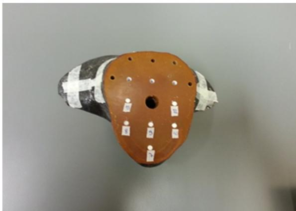
*Fig. 3.* The TLD chips inserted in their holes (from 1 to 6) in the slice, which was then fitted into the RANDO phantom.
