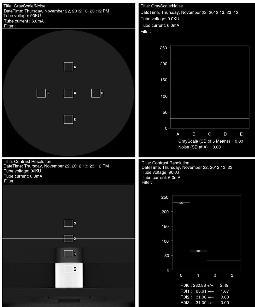
**Fig. 7.** Contrast measurement in 3D Accuitomo 80 (60 × 60, 90 kV, 6 mA) showing the uniformity/grayscale of five selected regions in the phantom (upper left panel), and the SD value of their five means besides the SD of the noise at the central region (upper right panel). The contrast resolution using four different materials in the phantom (lower left panel) was tested and the values are shown in the graph (lower right panel).
