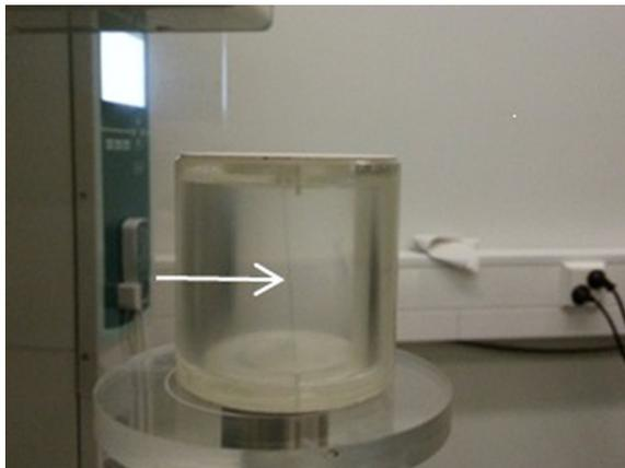
*Fig. 2.* A wire phantom, with the wire appearing vertical in the middle of the cylinder (arrow).
