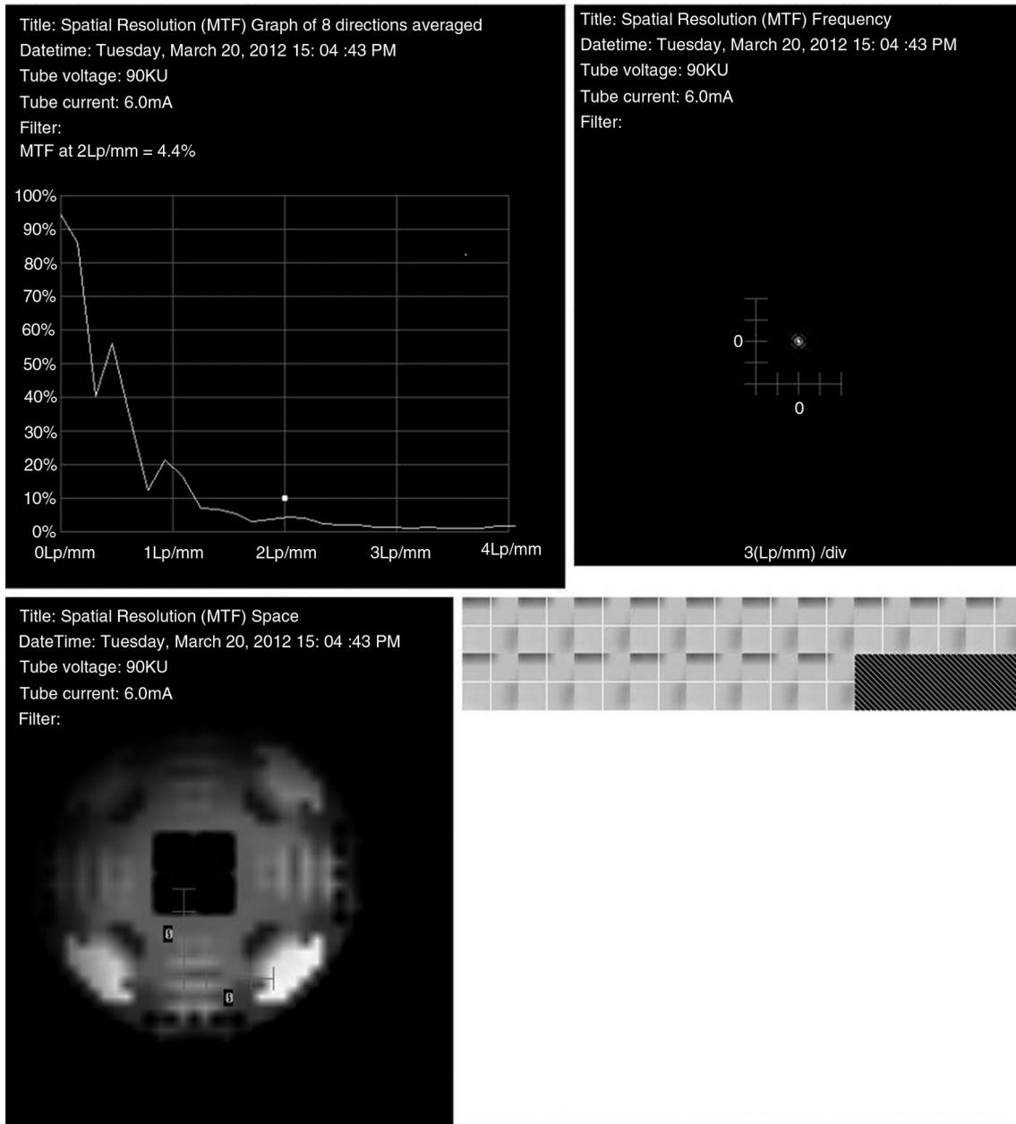
**Fig. 4.** MTF graph in 3D Accutomo 80 ( $60 \times 60$ , 90 kv, 6 mA) to be 4.4% when set at 2 lp/mm (upper left panel). The object on which MTF value was assessed had a spatial frequency of 3 lp/mm (upper right panel) in the space inside the phantom (lower left panel). Axial slices of the object show the luminance intensity after receiving the X-ray signal; no artifacts were noticed (lower right panel).
