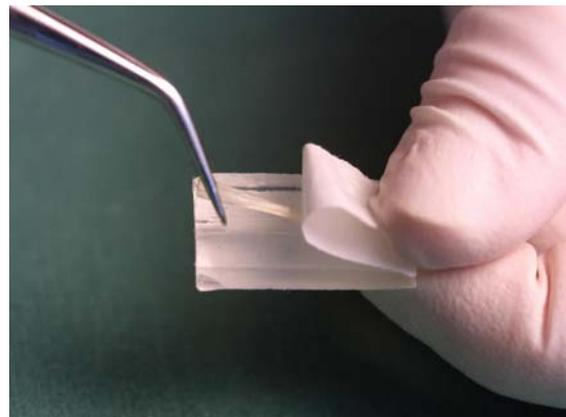
Figure 3. Preimpregnated fiber reinforced composite
