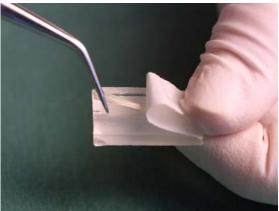
Figure 3. Preimpregnated fiber reinforced composite
