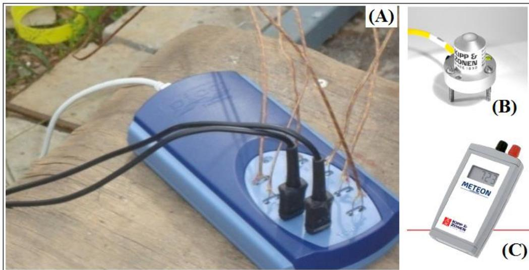
Figure 7. A) USB TC-08 data logger, B) SP LITE Silicon Pyranometer and C) Radiation data logger.
