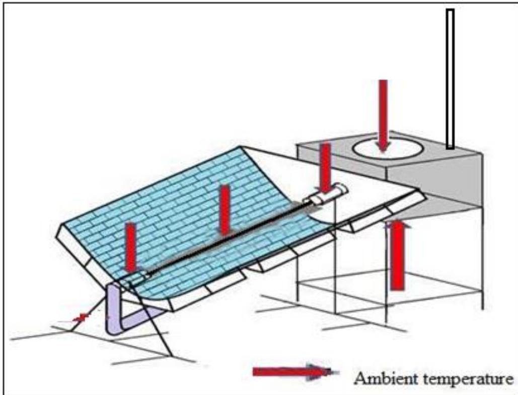
Figure 6. A schematic of the main components and temperature measuring points.
