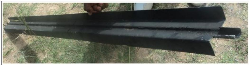
Figure 4. Folded aluminum plate, coated with ABRO black.
