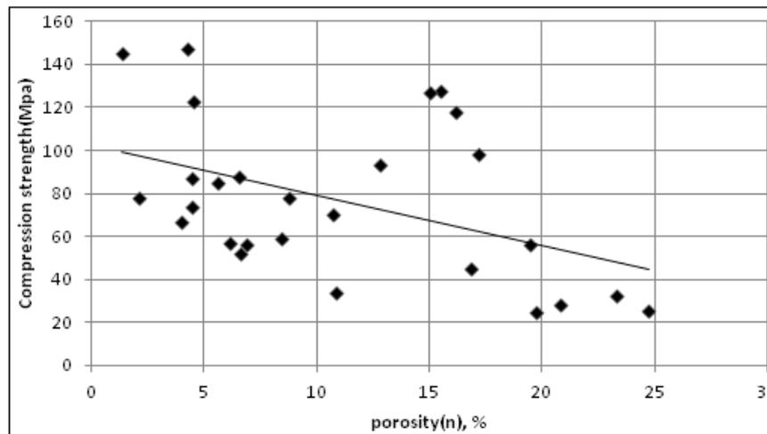
Figure 7. Compression strength as a function of total porosity.
