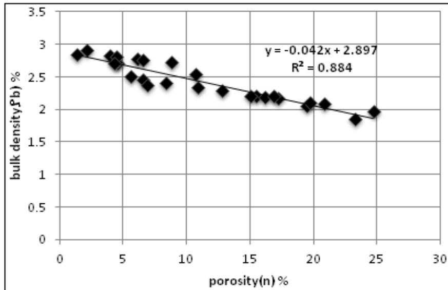
Figure 5. Graph showing Porosity versus bulk density.
