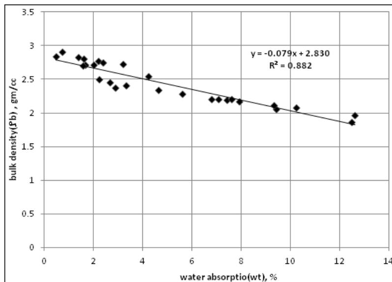
Figure 6. Water absorption versus bulk density.
