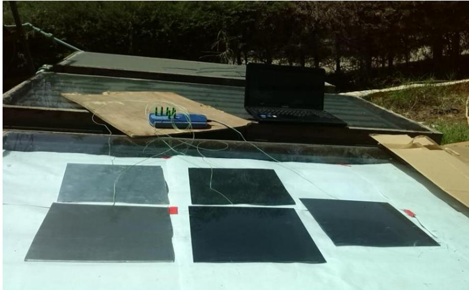
Figure 1. Flat plate specimen of aluminum and iron sheet metals.
