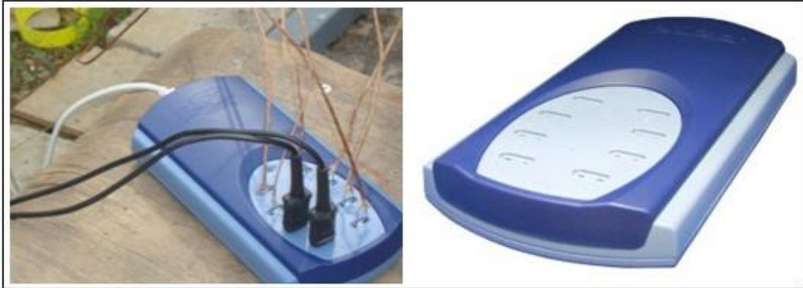
Figure 4. Temperature measuring USB TC-08 data logger.
