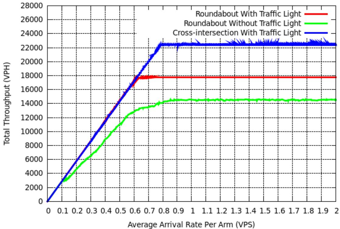
Figure 6. Comparison of roundabout without traffic light, roundabout with traffic light and cross intersection. The figure shows the comparison of roundabout with traffic light and cross intersection. In the simulation the light is assumed to be red for 40 seconds and green for 20 seconds. The yellow time is assumed to be 2 seconds. Every other assumption discussed in this paper also hold true.
