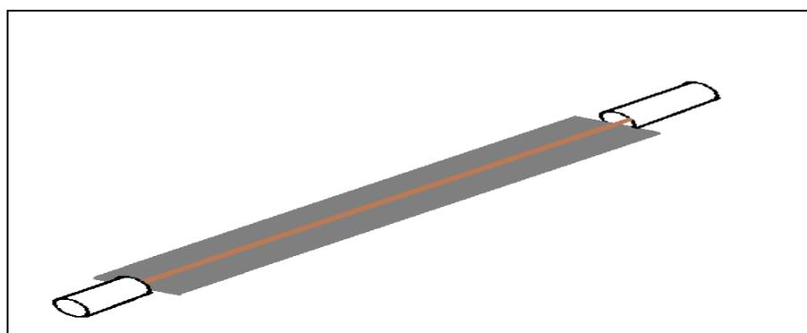
Figure 2. Copper tube in a corrugated aluminum sheet.
