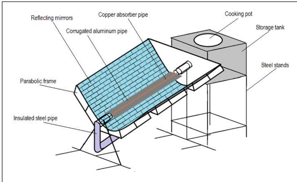
Figure 1. Sketch assembly of the solar cooker.
