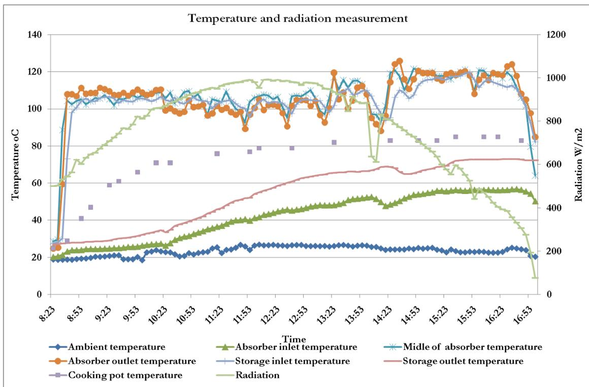
Figure 9. Radiation and temperature measured on 21<sup>st</sup> October 2010.
