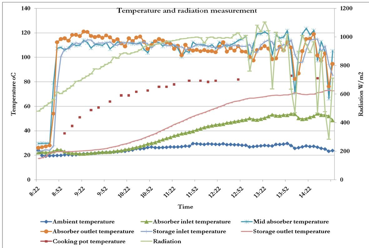
Figure 8. Radiation and temperature measured on 19<sup>th</sup> October 2010.
