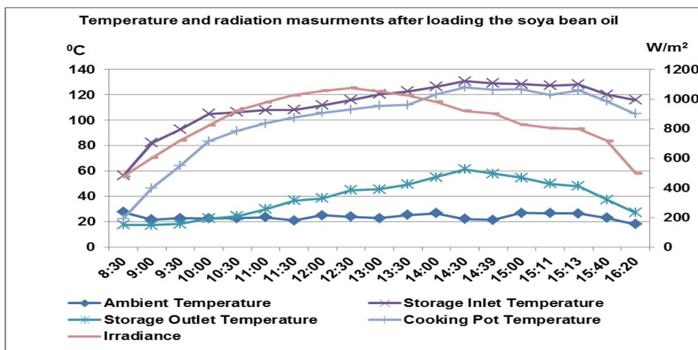
Figure 13. Radiation and temperature measured on 22<sup>nd</sup> March 2011.
