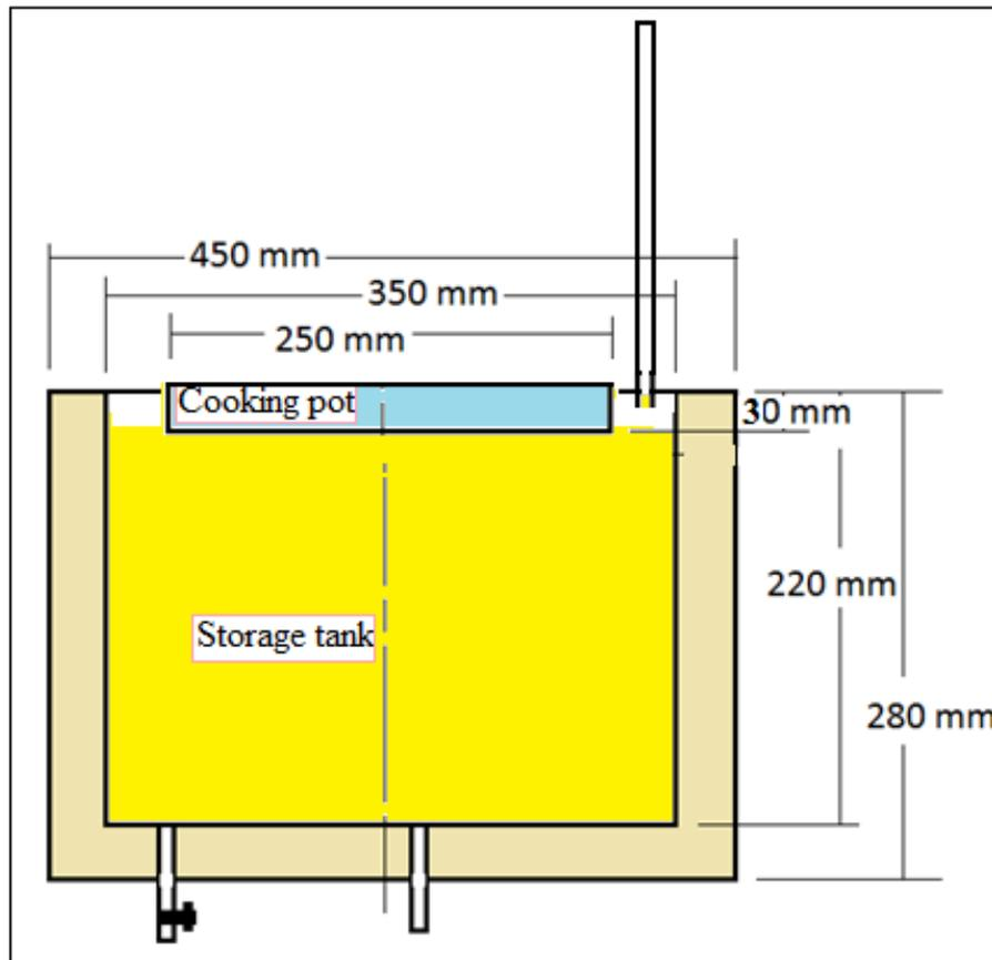
Figure 5. The modified storage tank and cooking pot.
