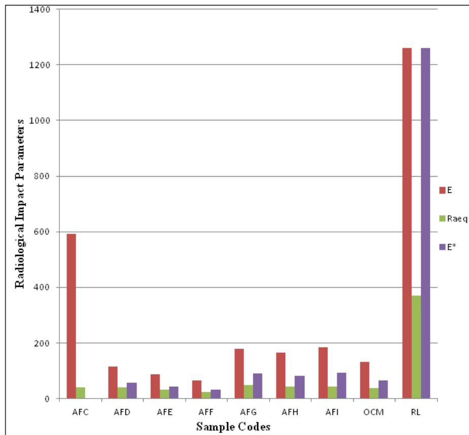
Figure 2. Radiological impact parameters for tobacco products(UNSCEAR, 2000). (Note: D is the absorbed dose rate; E is the equivalent dose for 100 % of the smoke: Raeq is the radium equivalent activity index and E\*is the equivalent dose for 50 % of the smoke inhaled by primary smoker; and RL is the world average values).
