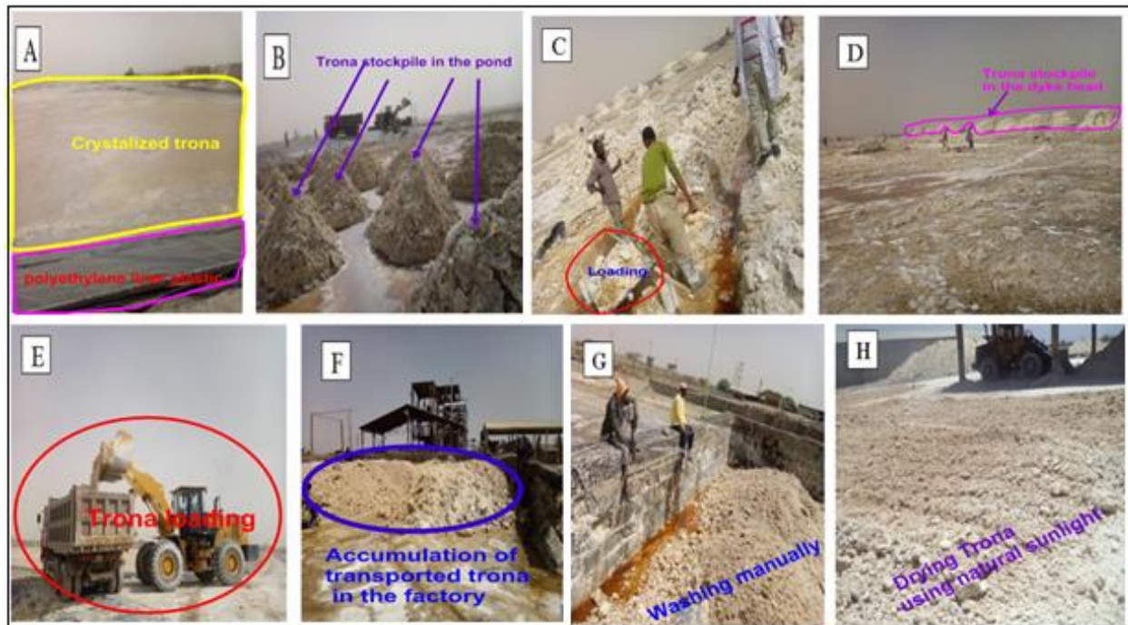
Figure 1. Photographs showing trona production process, starting from trona crystallization to the processing plant, A) crystallized trona, B) harvesting and stockpile trona in the pond, C) removing trona from the pond, D) accumulating trona in the dyke head, E) loading trona from the head dyke, F) piling (accumulating) trona for washing, G) washing trona manually by groundwater, and H) drying washed trona by sunlight.
