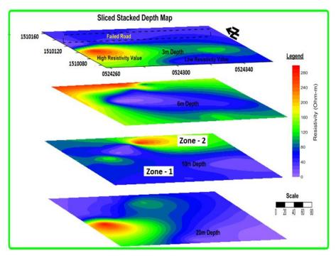
Figure 6. Apparent resistivity sliced-stacked depth map at various depth levels at half electrode separation (AB/2).
