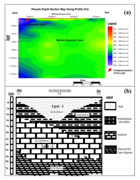
Figure 7. (a) Apparent resistivity pseudo-depth section map along profile 1 (b) geo-electric section map along the road failure.
