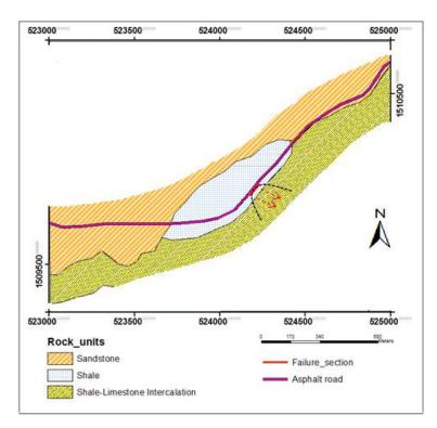
Figure 2. Geological map of the study area and its surrounding. The black dashed line indicates affected zone and dashed arrows show sliding direction of the landslide.
