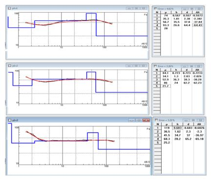
Figure 5. Interpreted VES curves of the three sounding points along the road failure.
