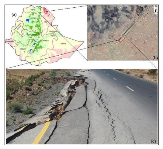
Figure 1. (a) Digital elevation map of Ethiopia (b) Google image of Mekelle – Abi-Adi road segment (c) road failure of the study area.
