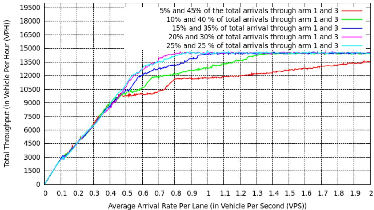
Figure 4. The effect of unbalanced traffic flow at the entrance of a double-lane roundabout. This figure shows the effect of unbalanced traffic volume at entrance road of a roundabout on performance. In this figure traffic volume at arms 2 and 4 are assumed to be each 25% of the total. The rest 50% is distributed unequally to arms 1 and 3 as indicated in the legend.
