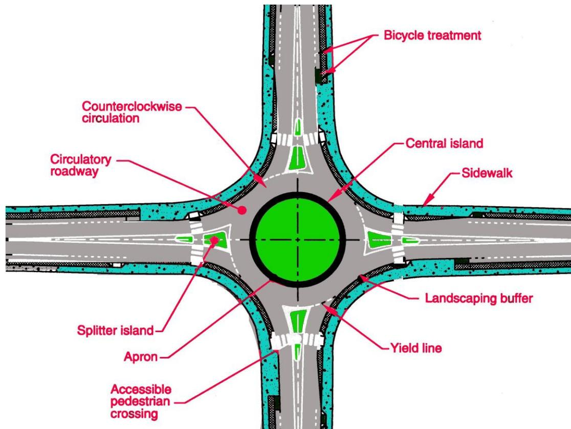
Figure 1. A roundabout with four arms describing the physical geometric design (from Robinson et al., 2000).
