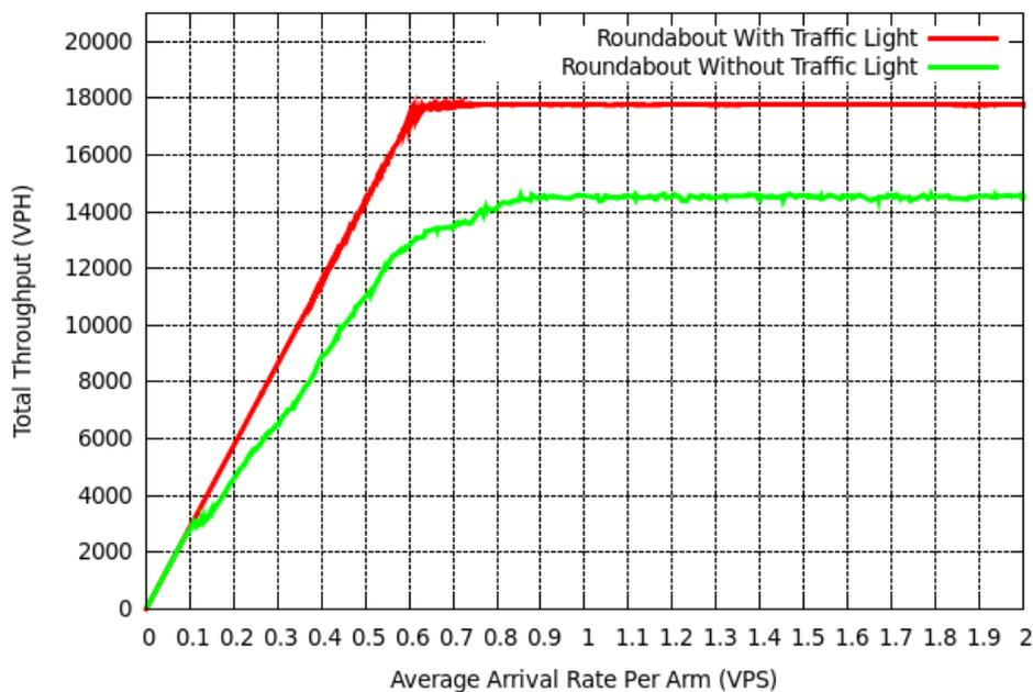
Figure 5. Comparison of roundabouts with and without traffic light. The figure shows the comparison of roundabout with and without traffic light. In the simulation the light is assumed to be red for 40 seconds and green for 20 seconds. Theyellow time is assumed to be 2 seconds. All other assumptions discussed in this paper also hold true.
