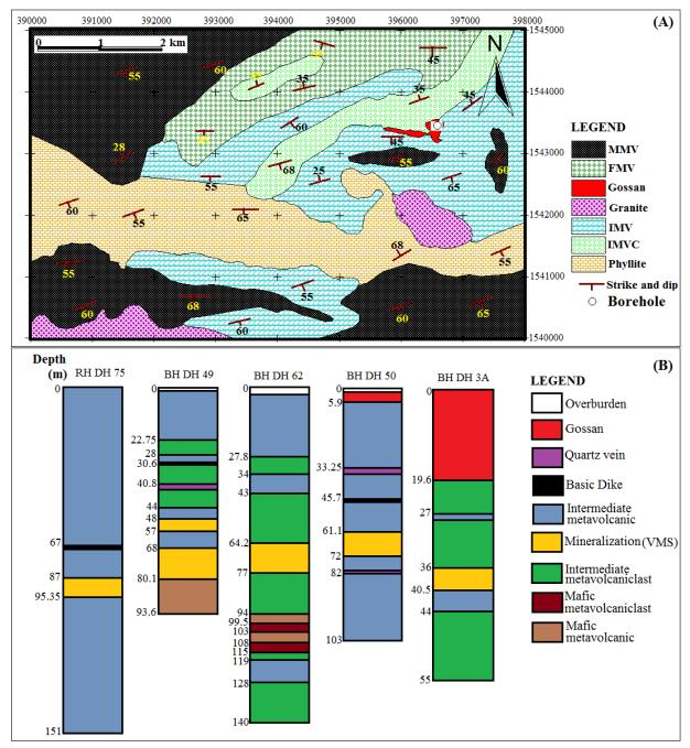
Figure 2. (A) Geological map of the study area (after Bheemalingeswara and Atakilt, 2012) and (B) drill core logs of five boreholes.
