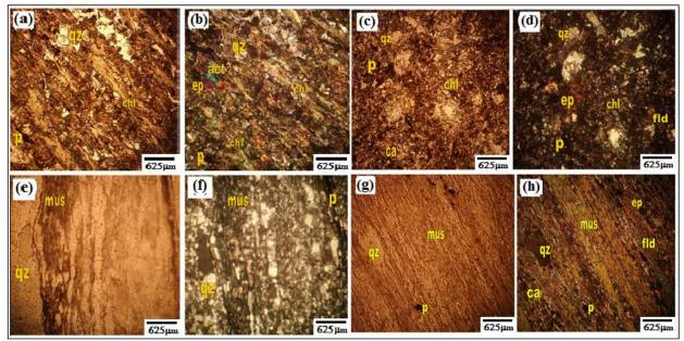
Figure 3. Microphotographs of (a) mafic metavolcanic rock (PPL) and (b) XPL; (c) intermediate metavolcanic rock (PPL) and (d) XPL; (e) metavolcaniclastic rock (PPL) and (f) XPL; and (g) phyllite (PPL) and (h) XPL [qz=quartz, chl=chlorite, act=actinolite, ca=calcite, kfld=k-feldspar, fld=feldspar, bt=biotite, mus=muscovite, ep=epidote, p=opaque].
