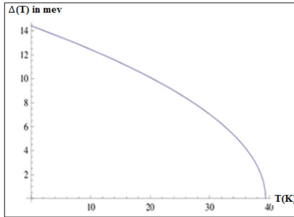
Figure 2. Transition temperature ( $T_C$ ) versus superconducting order parameter ( $\Delta$ ) for  $Ba_{1-x}K_xFe_2As_2$  superconductor.
