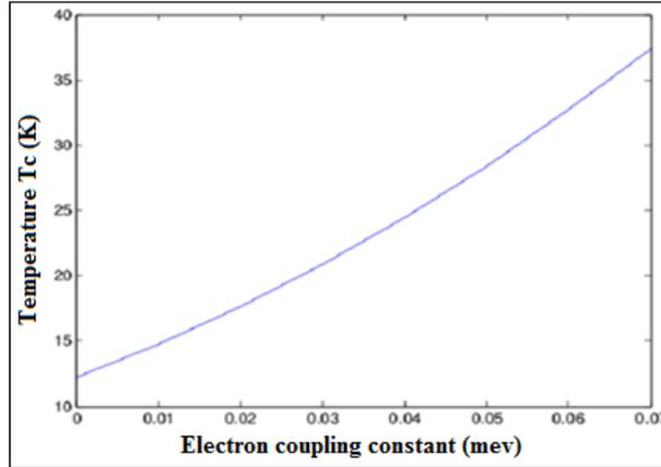
Figure 1. Electron coupling constant ( $\lambda_{el}$ ) versus superconducting temperature ( $T_C$ ) for  $Ba_{1-x}K_xFe_2As_2$  superconductor.
