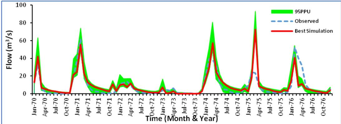
**Figure 3:** Calibration results for average monthly streamflow.
