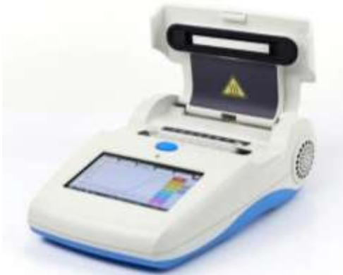
**Figure 4:** The Genie II instrument for real-time LAMP. This instrument can be portable and run from a battery. The method is ideally suited for non-research laboratories that need to fulfil a limited number of diagnostic tests on a regular basis
