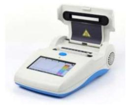
**Figure 4**: The Genie II instrument for real-time LAMP. This instrument can be portable and run from a battery. The method is ideally suit for non-research laboratories that need to fulfil a limited number of diagnostic tests on a regular basis
