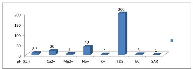
Fig. 2: FAO Permissible value for irrigation water
