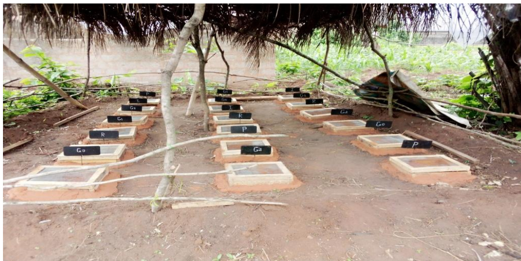
Figure 4: Complete layout of the underground clay-composite storage chambers Mass loss profile for different pits
