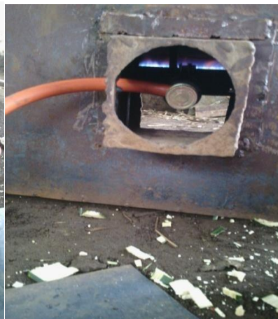
Plate 2: Heat supply to pyrolyser chamber
