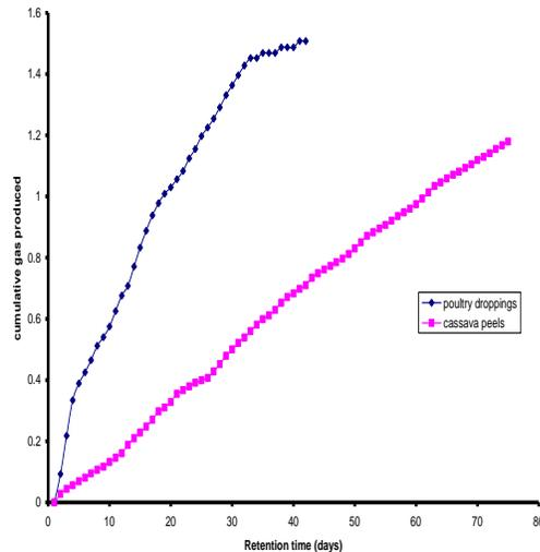
Fig. 6: Cumulative biogas generation during fermentation
