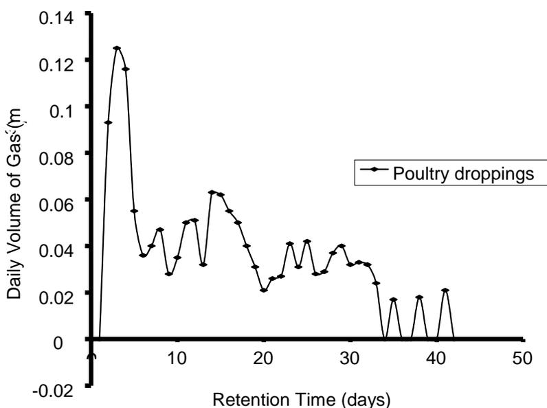
Figure 1: Effect of Retention Time on Biogas production
