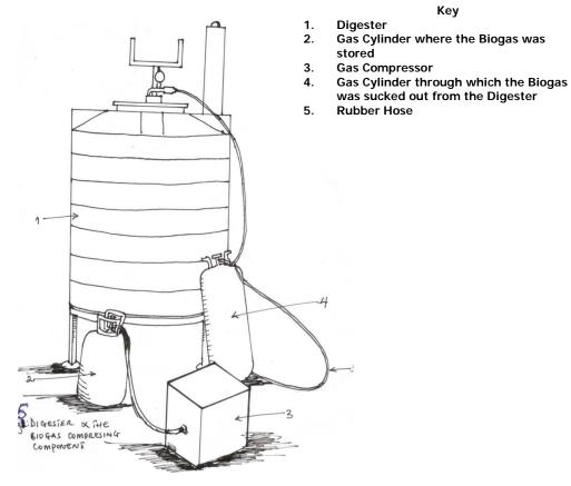
Fig. 2a: Digester & the Biogas Compressing Component
