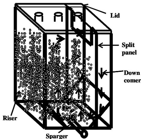
Fig.1. A multi-purpose airlift bioreactor for enzyme and yeast inoculum production.
