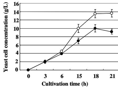
Figure 4. Comparison of yeast seed culture production in flask (●) and the constructed bioreactor (○) with an initial glucose concentration of 50 g/L
