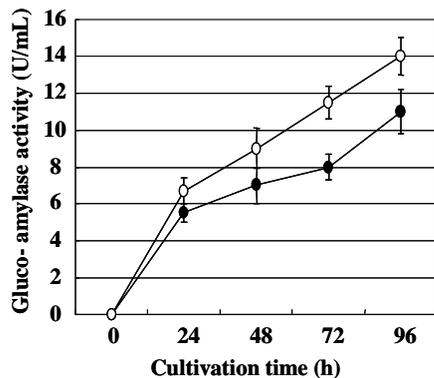
Figure 3. Comparison of gluco amylase production in flask (●) and the constructed bioreactor (○).
