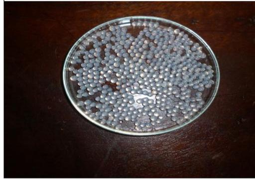
**Fig. 1. Alginate gel beads**
