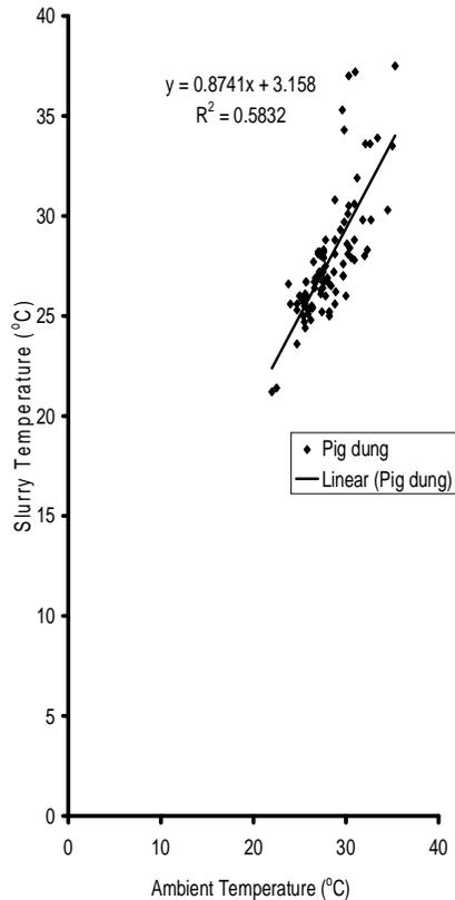
**Fig 4:** Maximum Ambient versus Slurry Temperature
