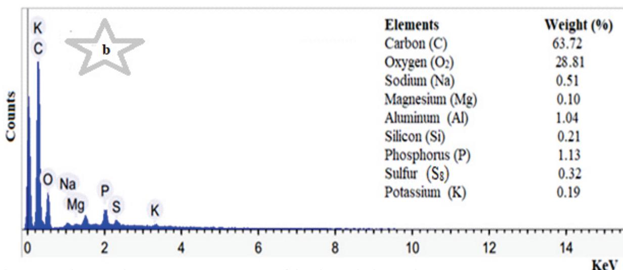
**Figure 3:** Elemental composition spectrum of the degraded sample
