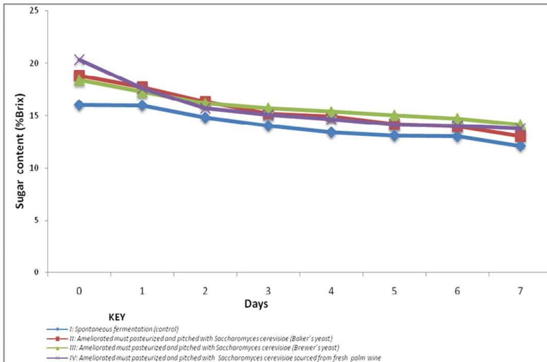
Figure 5: Changes in Sugar Content (% Brix) associated with fermentation of soursop must to wine at  $26 \pm 2$  °C.
