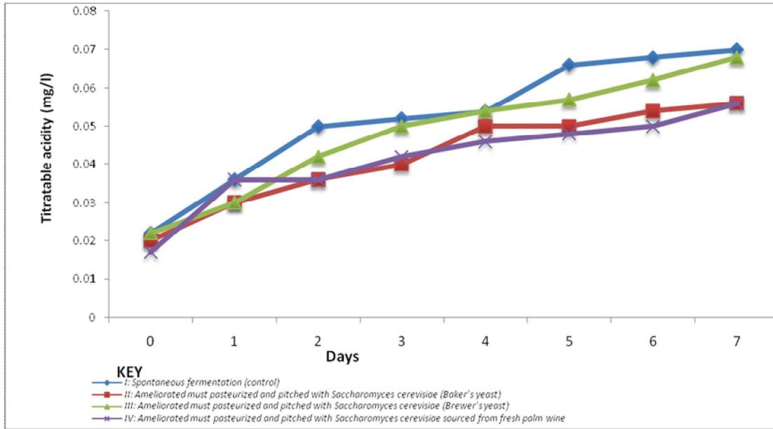
Figure 2: Changes in Titratable Acidity Values associated with fermentation of soursop must to wine at  $26 \pm 2^{\circ}\text{C}$ .
