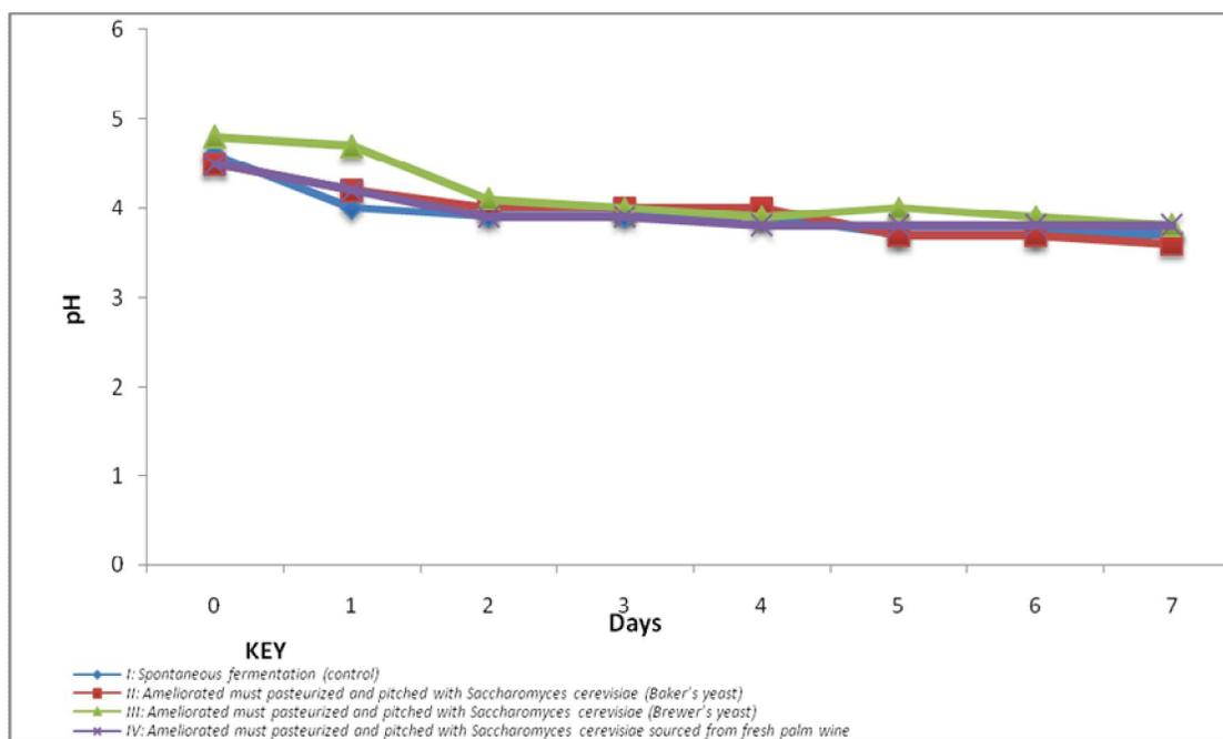
Figure 1: Changes in pH Values associated with fermentation of soursop must to wine at  $26 \pm 2$  °C.
