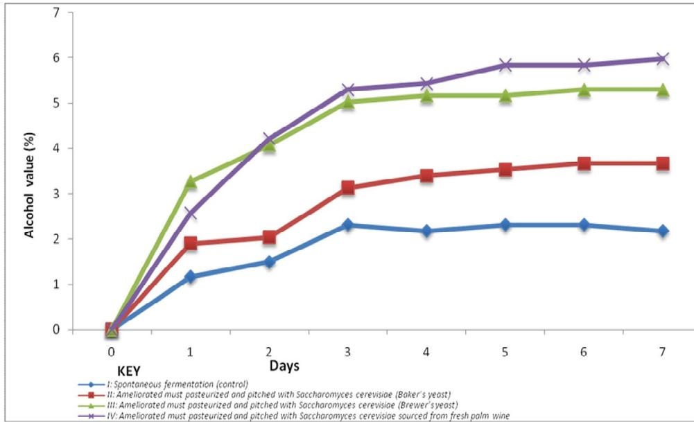
Figure 4: Changes in Alcohol Content (%) associated with fermentation of soursop must to wine at  $26 \pm 2$  °C.
