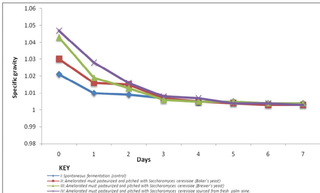
Figure 3: Changes in Specific Gravity associated with fermentation of soursop must to wine at  $26 \pm 2^{\circ}\text{C}$ .
