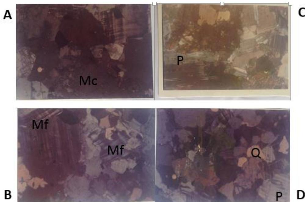
Figure 4. Petrography of some of the rocks in the study area (magnification x40): A and B represent migmatite-gneiss rocks; C = Diorite; D = Granite. Mc = muscovite; Mf = Microcline feldspar; P = Plagioclase; Q = Quartz
