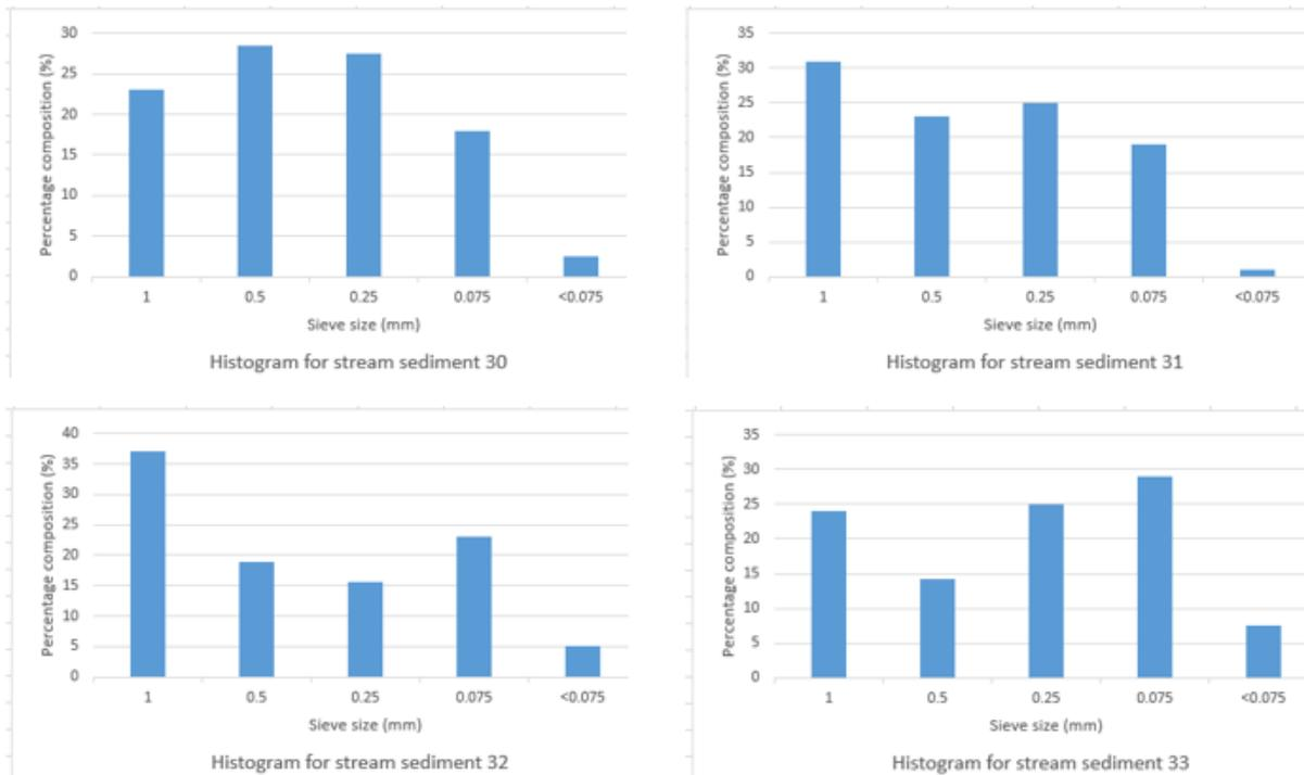
**Figure 5.** Histogram plots of the grain size analysis of the selected stream sediments in the area. The predominant grain sizes is 0.25 – 0.5 mm indicating coarse – very coarse grained deposits; the least common grain size is <0.075 – 0.075 mm.
