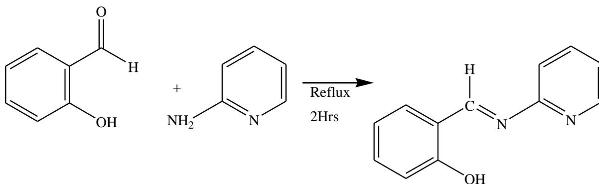
**Scheme 1:** Preparation of N-(2-hydroxylbenzylidene) Pyridine-2-amine
