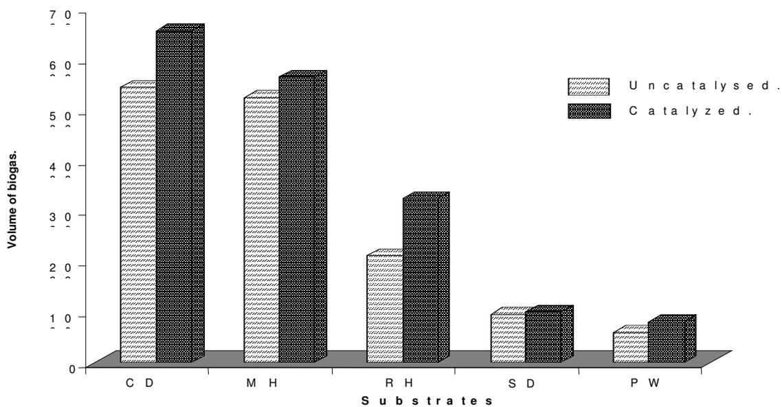
**Figure 5:** Cumulative volumes of biogas produced for both the catalyzed and uncatalyzed slurries.
