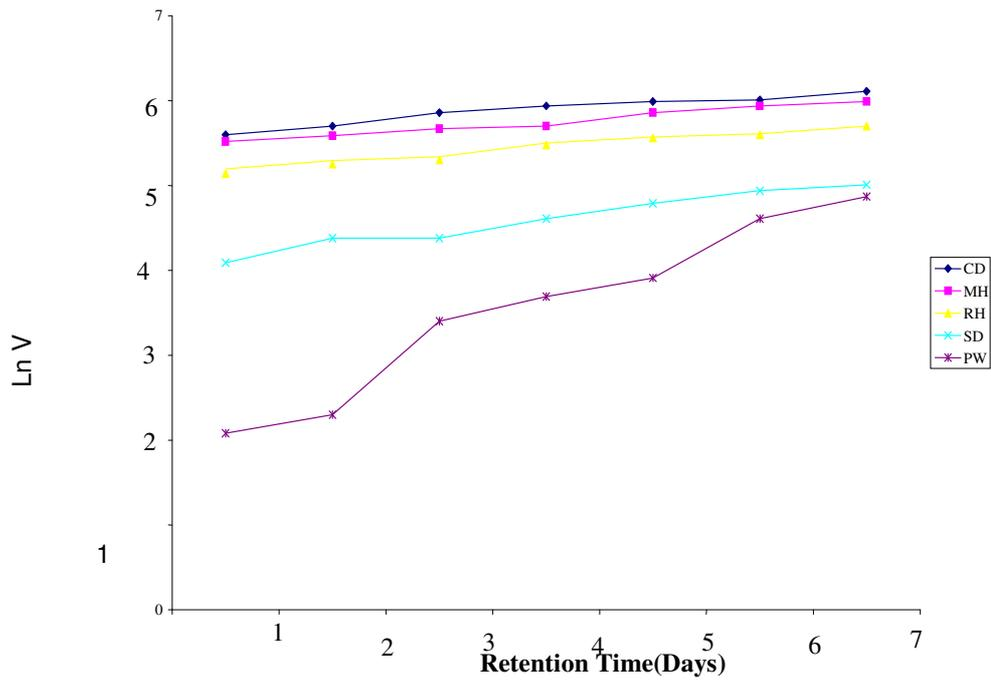
**Figure3:** plots of Ln V against time for the uncatalyzed bioconversion of the substrates
