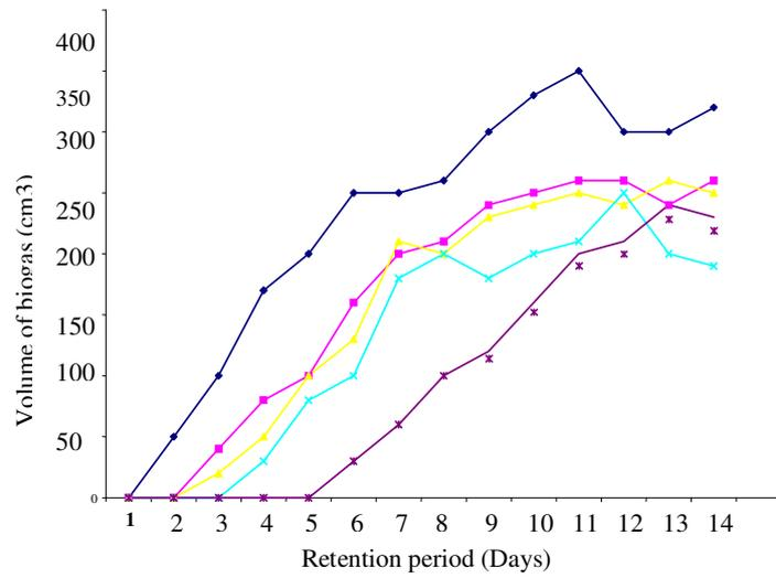
**Figure 2:** uncatalyzed biogas production in the first two weeks of the retention period.
