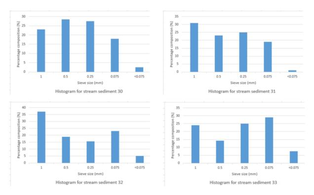
**Figure 5**. Histogram plots of the grain size analysis of the selected stream sediments in the area. The predominant grain sizes is 0.25 - 0.5 mm indicating coarse – very coarse grained deposits; the least common grain size is < 0.075 - 0.075 mm.
