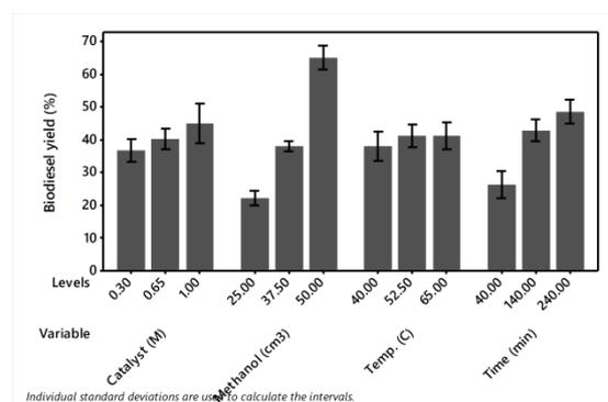
**Figure 1.** Mean effect of the reaction variables on the yield of biodiesel from *Jatropha* seed oil.
