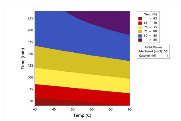
**Figure 2.** Contour plot of the effect of reaction time and reaction temperature on the yield of biodiesel from *Jatropha* seed oil
