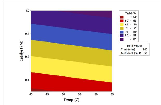
**Figure 4.** Contour plot of the effect of catalyst concentration and reaction temperature on yield of biodiesel from *Jatropha* seed oil.
