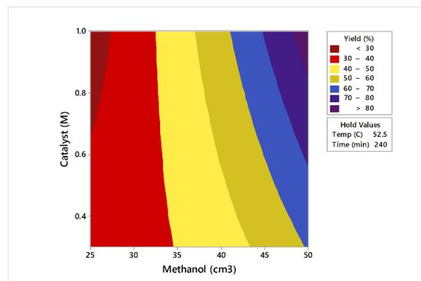
**Figure 7.** Contour plot of the effect of catalyst concentration and amount of methanol on the yield of biodiesel from *Jatropha* seed oil
