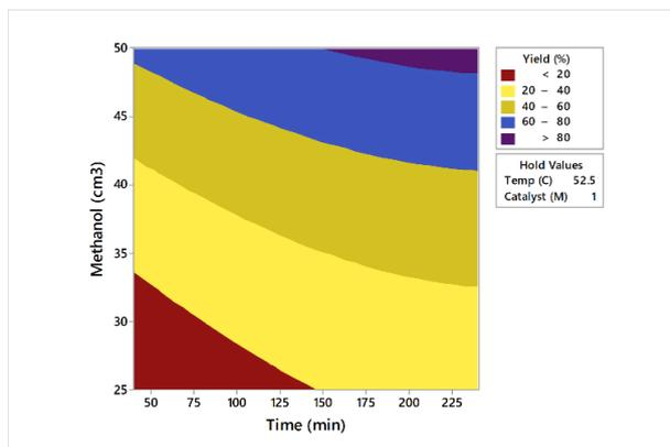
**Figure 5.** Contour plot of the effect of the amount of methanol and reaction time on the yield of biodiesel from *Jatropha* seed oil.
