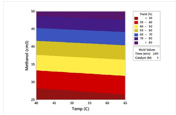
**Figure 3.** Contour plot of the effect of the amount of methanol and reaction temperature on the yield of biodiesel from *Jatropha* seed oil
