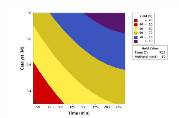
**Figure 6.** Contour plot of the effect of catalyst concentration and reaction time on the yield of biodiesel from *Jatropha* seed oil
