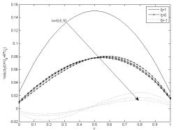
**Figure 6**: Variation of velocity (U) for different value of  $In \ (R = 0.05, \beta_v Kn = 1.667)$
