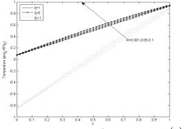
**Figure 3**: Variation of temperature  $(\theta)$  for different value of *R* and  $\xi$  $(\beta, Kn = 0.05, In = 1.667)$
