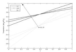
**Figure 7**: Variation of temperature ( $\theta$ ) for different value of *In* (*R* = 0.05,  $\beta$ . *Kn* = 1.667)
