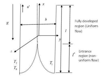
Figure 1: A schematic geometry of natural convection flow in a vertical parallel plate micro-channel
