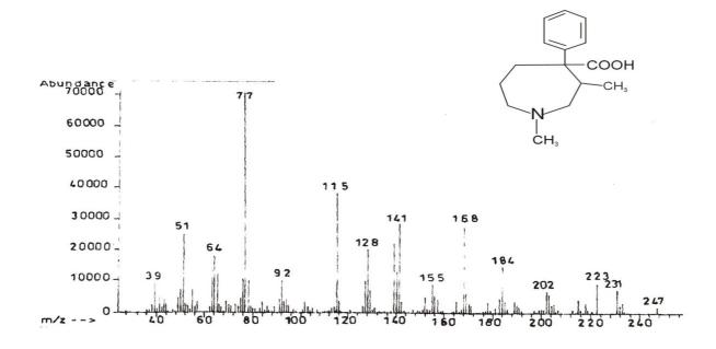
Figure 2: Mass spectrum of hexa hydro -1,3 - dimethyl -4- phenyl -IH- azepine -4- carboxylic acid
