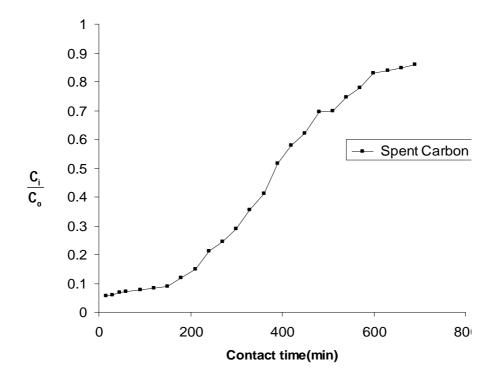
Figure 2: Breakthrough curve for the adsorption of Methyl Red onto Commercial Activated Carbon
