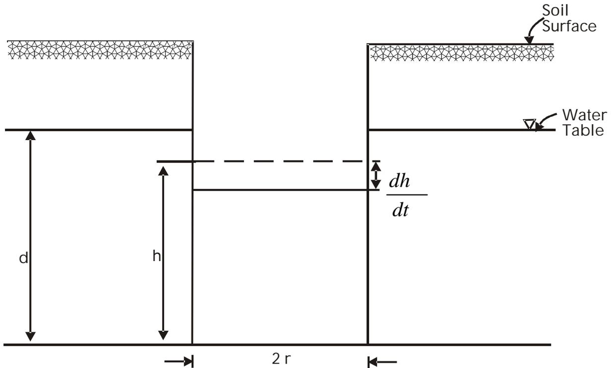
Figure 2: A schematic presentation of the auger-hole technique
