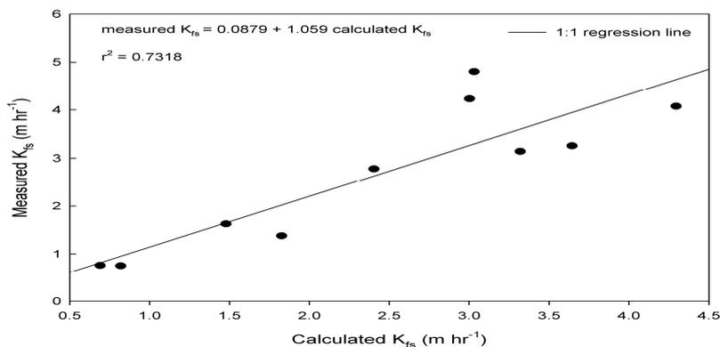
**Figure 3:** Measured and calculated field saturated hydraulic conductivity from effective porosity of 30-45cm soil depth
