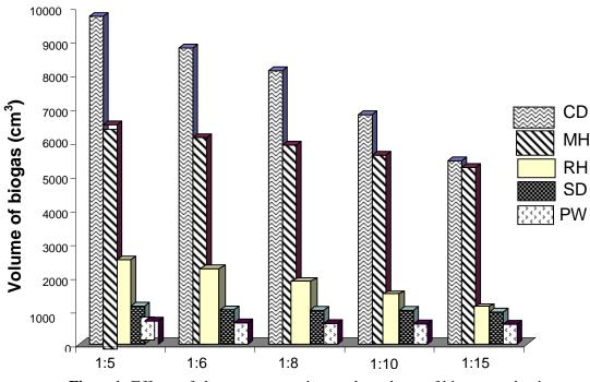
Figure1: Effects of slurry concentration on the volume of biogas production.
