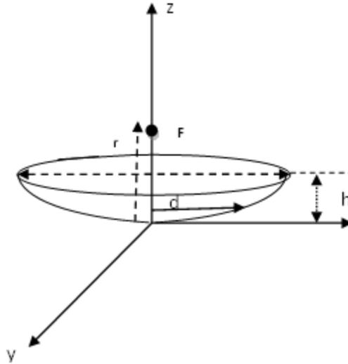
Figure 1: Schematic diagram of parabolic solar dish
