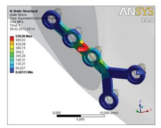
Figure 7: Three-dimensional Von Mises stress distribution fields in Y plate
