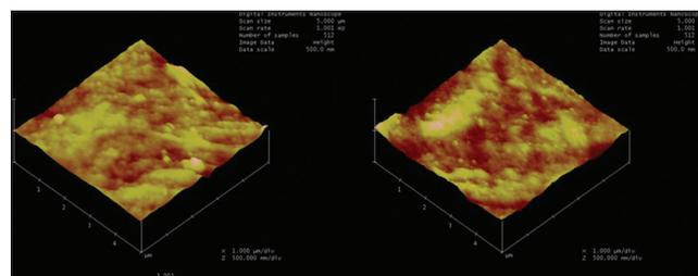
**Figure 1:** Three-dimensional atomic force microscopy images of new and used Twisted Files 25.06 instruments
