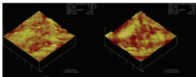
**Figure 1:** Three-dimensional atomic force microscopy images of new and used Twisted Files 25.06 instruments
