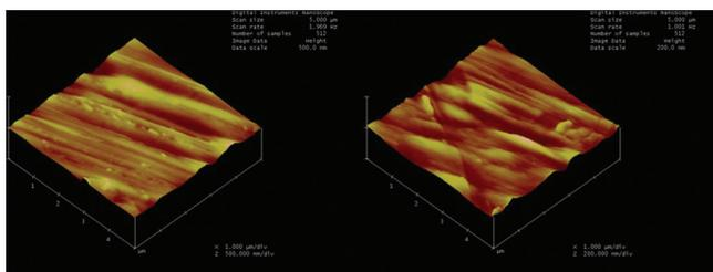
**Figure 2:** Three-dimensional atomic force microscopy images of new and used Mtwo 25.06 instruments
